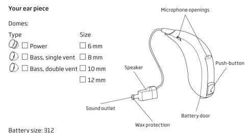
Open the battery door fully to allow air to circulate whenever you are not using your hearing instrument, particularly overnight.
