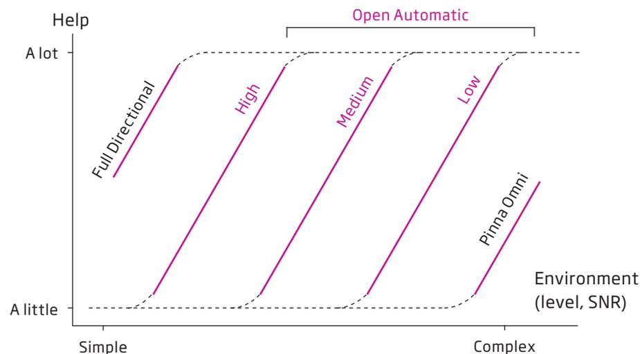
OSN directionality settings. In Pinna Omni, the hearing aid mimics sound as received by the human ear. In Full Directional, the focus is on sounds coming from the front. In Open Automatics, the hearing aid automatically adapts to the acoustical conditions, based on one of the three help profiles, High, Medium, or Low.
