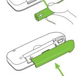
(i) The mini-USB port cannot be used for battery charging. Do not use rechargeable batteries.
