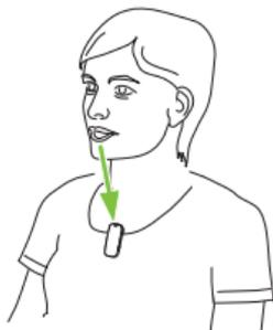
① The greater the surrounding noise, the closer the RemoteMic should be positioned to the speaker's mouth.
